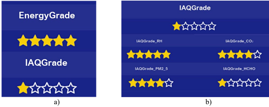
Fig. 5. Post-processor window: a) EE and IAQ grades and b) IAQ grade by type of pollutant for a specific configuration.
